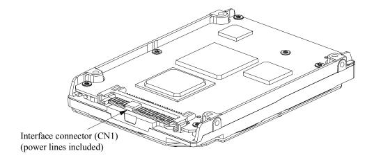
Figure 4.9 Connector location
